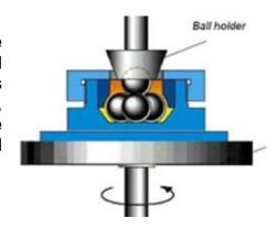
Most Product Data Sheets will list the weld point, but there are two other observations that are also commonly recorded for the EP test: Last Non-Seizure Load (LNSL) and Lubricant Wear Index (LWI).
