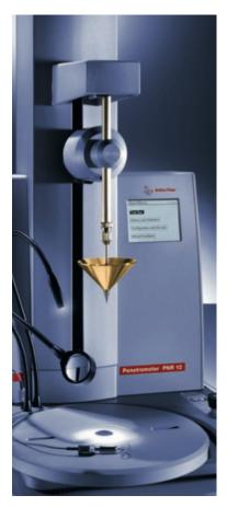
"Penetration" refers to the depth to which a cone penetrates a cup of the subject grease in a penetrometer during a specified period of time. Cone penetration tests provide one measure of the consistency of a grease.
