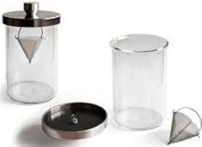
There are several standardized procedures for measuring the degree to which oil separates from the thickeners and additives in lubricating grease. Each test is designed for a different purpose; measuring the effects of centrifugal force (for grease in couplings and u-joints for example), measuring separation during storage (in 35 lb. kegs), and for testing separation for quality control and specification purposes.
