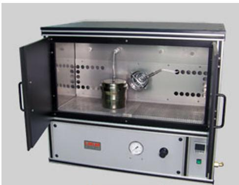
Significant oil separation may or may not be a desirable characteristic of the grease, depending on its application. For example, if a significant amount of oil separates, the percentage or level of thickener or additives left in the grease may change which may or may not be desirable. Or, separation of some oil from the grease may allow the base oil in the grease to flow into otherwise inaccessible surfaces.
